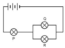
The filament of bulb **R** breaks. Which ONE of the following correctly shows the CHANGE IN POTENTIAL DIFFERENCE across bulbs **P** and **Q**?
