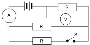
Switch **S** is now closed. Which ONE of the following combinations correctly gives the changes in the readings on the ammeter and voltmeter?
